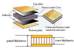
Fig.1.1: Honeycomb sandwich panel
