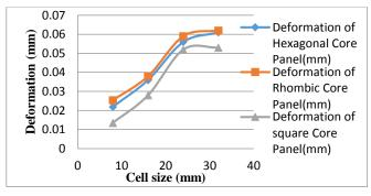
Fig.5.7: Deformation of honeycomb panel with varying cell size
