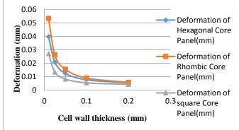
Fig.5.5: Deformation of honeycomb panel with varying cell wall thickness
