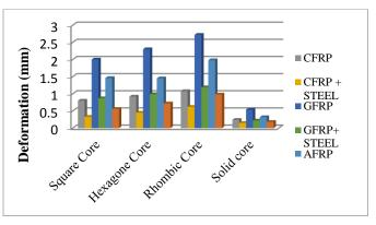
Fig.5.11: Comparison of deformation of panel with different cores (Moving load)
