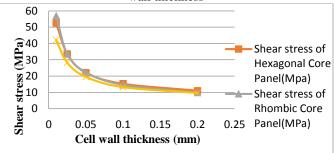
Fig.5.6: Shear stress of honeycomb panel with varying cell wall thickness
