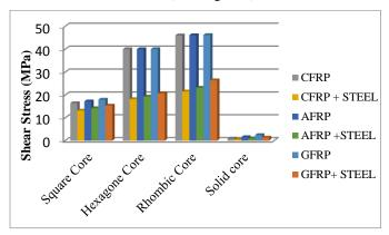
Fig.5.12: Comparison of Shear stress of panel with different cores (Moving load)
