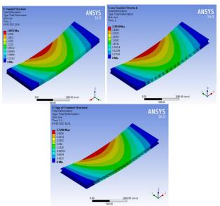
Fig.5.9: Deformation of square, hexagon and rhombic core GFRP panel in transient analysis
