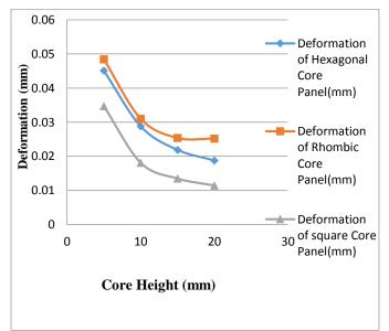
Fig.5.3: Deformation of honeycomb panel with varying core height
