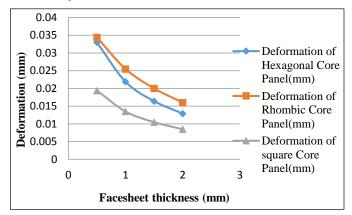
Fig.5.1: Deformation of honeycomb panel with varying face sheet thickness
